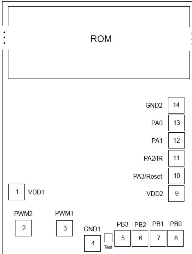
\* The IC substrate must be connected to GND or Floating.
